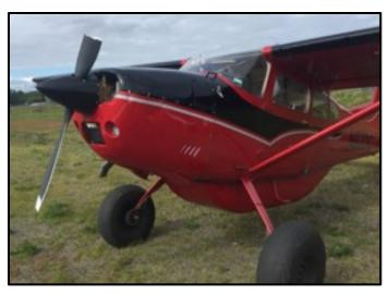
The airplane was equipped with a McCauley controllable pitch aluminum propeller, model number D2A34C58–0. An examination of the fractured blade revealed that it had failed due to fatigue cracking that initiated from a nick in the leading edge. Measurement of the nick revealed it was within tolerance for a field repair, although a field repair had not been performed. The NTSB determined that the
